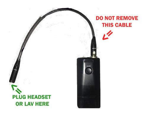
With the added wear and tear of repeated unplugging/plugging personal headset mics, some of these ports were getting damaged. It will be much easier and cheaper for us to replace the short sacrificial cable, than repairing/replacing the entire beltpack transmitter.
